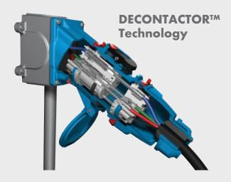
Pressing the pawl/button on the receptacle will safely switch off power to the load. The plug can then be withdrawn in complete safety.
