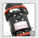
To disconnect, open the pilot circuit and unlock the plug by turning the ring until the "O" is aligned with the arrow. The power is now off.
