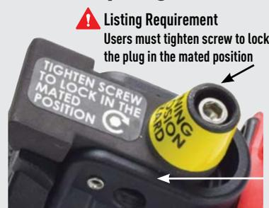
Zone 2/Division 2 DS60 receptacles feature a standard screw-type locking pawl. This required feature allows the user to lock the plug in the receptacle by tightening a screw on the pawl.
