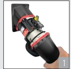
Before connection, ensure that the circuit is deenergized. Align the red dots, push the plug partially in, then turn clockwise slightly to line up the latch with the catch.
