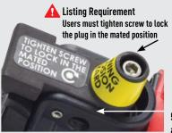
Zone 2/Division 2 DR50 receptacles feature a standard screw-type locking pawl. This required feature allows the user to lock the plug to the receptacle by tightening a screw on the pawl.
