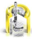
After depressing the pawl, the plug is rotated in a counterclockwise direction. This frees the switching contact for operation and the release of the remaining spring tension causes a quick breaking of the contacts. The plug may now be removed, if desired.
